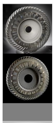
A good tire means a lot when the nearest roadside assistance is 34 million miles (55 million kilometers) away. For future rovers that will explore the surface of Mars, NASA scientists have created a tire that contains no air, can handle the rugged Martian terrain, and may even have applications on Earth for trucks and off-road vehicles.
