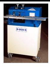
vertical edges of shaker parts in one pass. It eliminates "scallop" marks as it deburrs. Capable of deburring stainless steel, nickel and aluminum parts, this equipment will be essential to customers requiring a burr free edge for safe handling.
