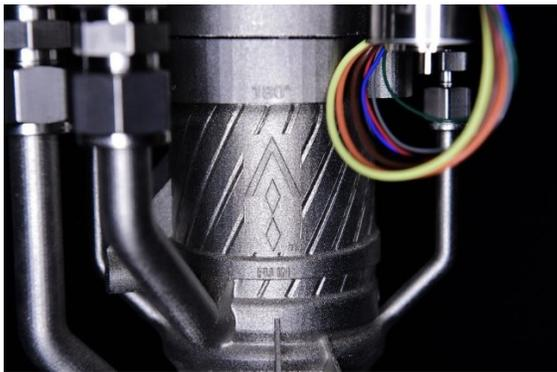
6K's Ni625 powder is being certified for use at Agile's manufacturing facility. The first parts to be produced will be used in Agile's A2200 bipropellant hypergolic engine. The engines are powered by a pressure-fed hypergolic bipropellant, which does not require ignition as the hydrazine derivative fuel, M20, and MON3 oxidiser combust on contact.
